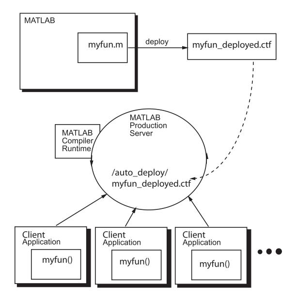
Deploying MATLAB code using MATLAB Production Server is a four-phase process:
